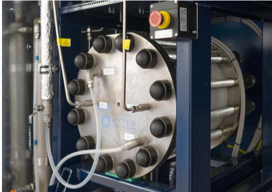
Figure 13 - Example of a Hyter AEM electrolyzer stack [11].
