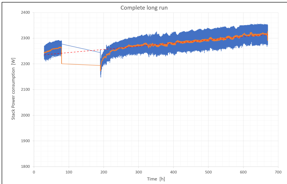
Figure 43 - Steady state nominal condition long run analysis. Dated back to 2021. In blue the original data shift. In orange the average value trend.
