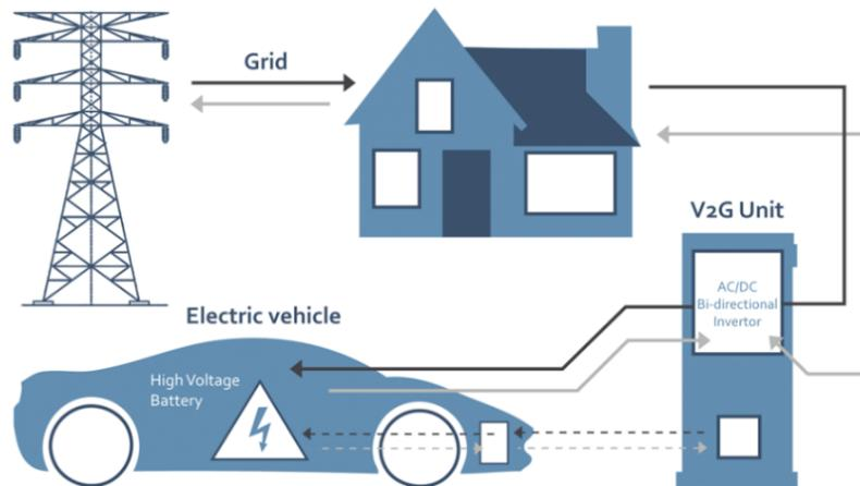
Figure 55: V2G power Exchange [35]
