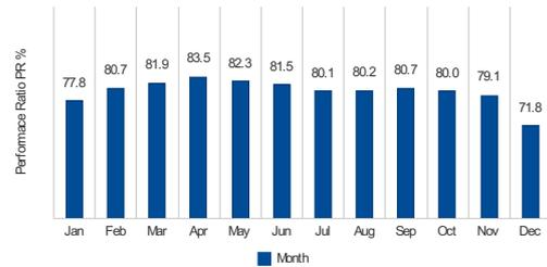
Figure 48: Simulation results of hotel swimming pool PV plant
