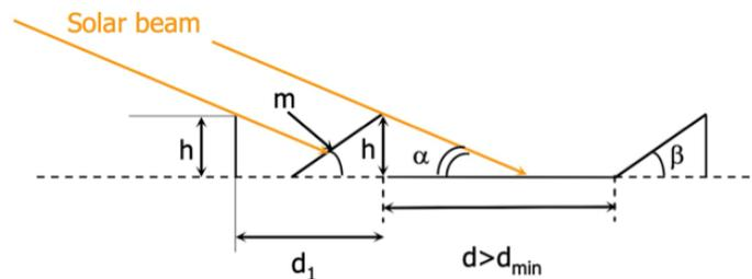
Figure 18: Solar beam angles and irradiation on photovoltaic modules
