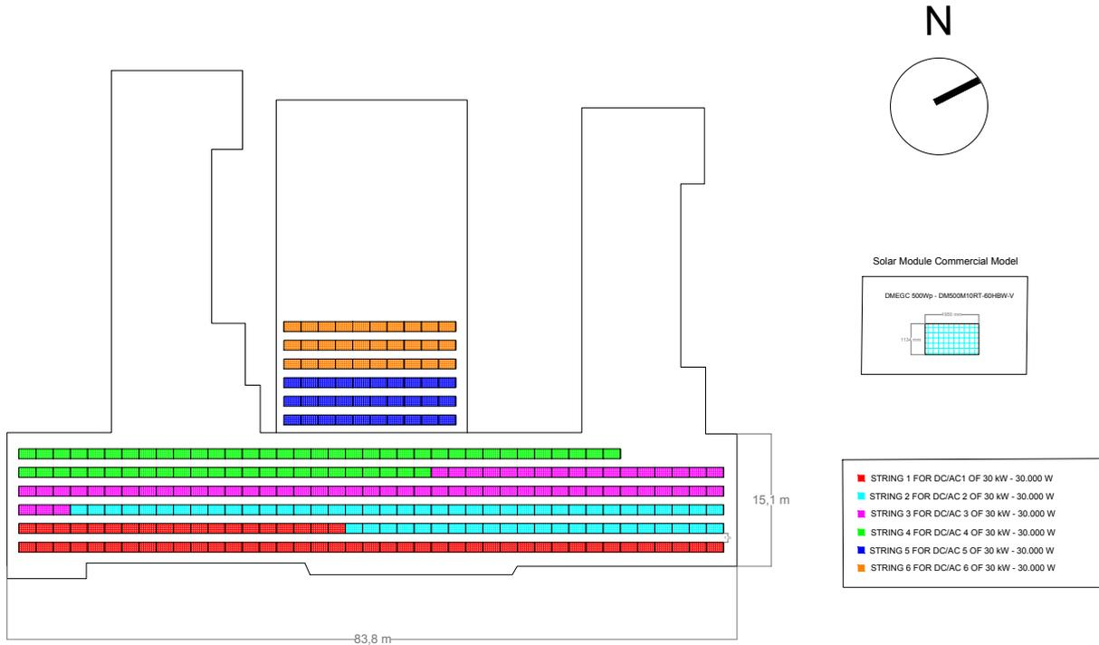
Figure 35: School photovoltaic layout in the optimized case
