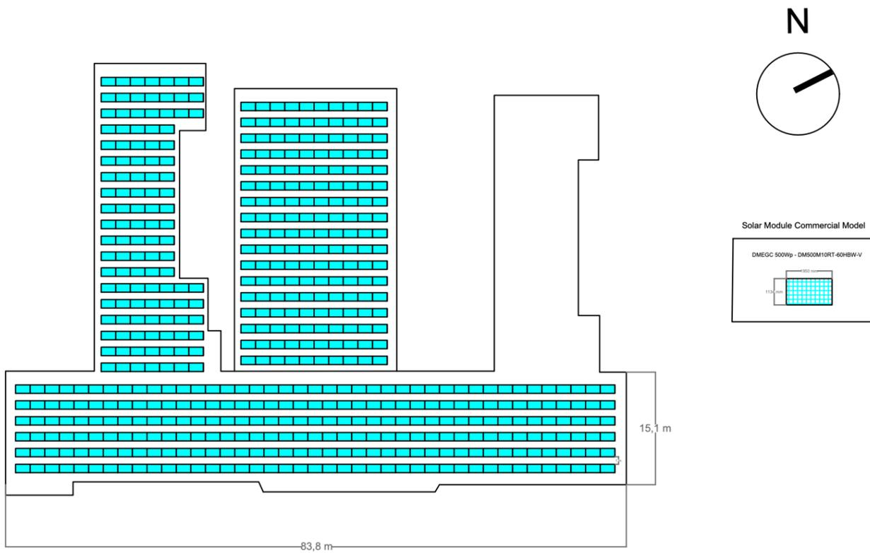
Figure 22: Solar photovoltaic layout on the school rooftop
