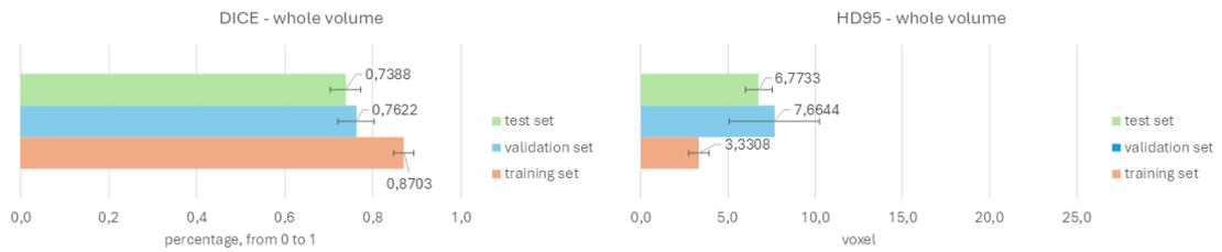
**Figure 4.13:** Whole volume metrics obtained with SwinUNETR 3D Neural Network with Generalized Dice Focal Loss function for thigh
