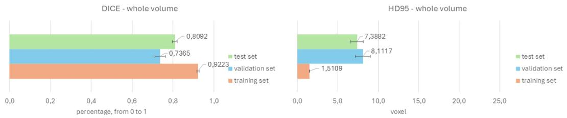
**Figure 4.22:** Whole volume metrics obtained with SwinUNETR 3D Neural Network with Focal Loss function for thigh
