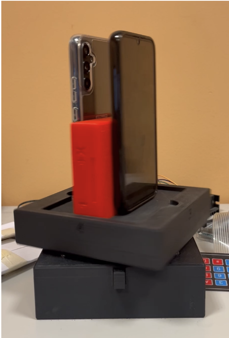
Figure 3.4: Rotating platform performing the 100 controlled rotations
