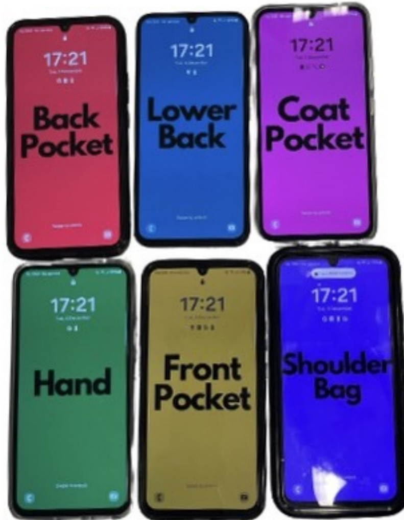
Figure 4.12: Customized smartphone backgrounds indicating their designated positions to ensure correct reattachment by participants.
