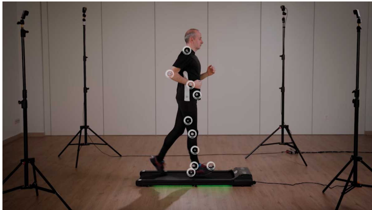
Fig. 1.5 Example of a marker-based optoelectrical motion capture system, from [5].
