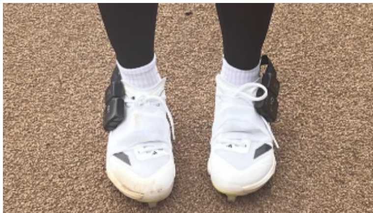
Fig. A.1 MIMUs placement on shoes dorsum, under the white tape; the black support refers to the pressure insole system.
