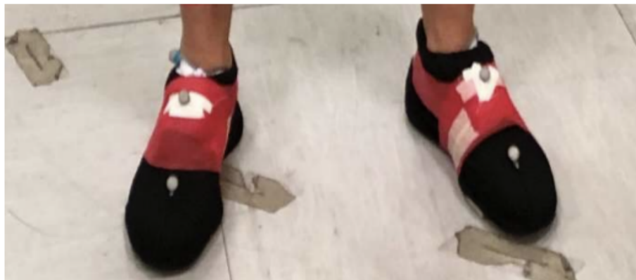
Fig. 3.2 Subject wearing MIMUs (under the red tape) together with retro-reflective markers (above the red tape).
