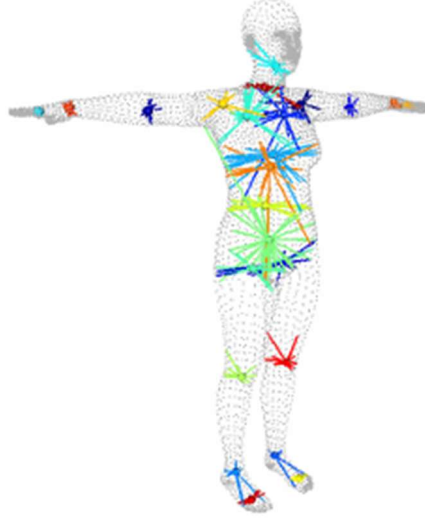
Figure 12: Estimation of joint centers positions. The left knee joint is computed as the weighted average of red vertices [47].
