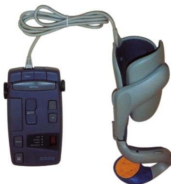
**Figure 2.3:** Handmaster system. The Handmaster consists of an external control unit connected via cable to a splint with integrated surface electrodes [55].
