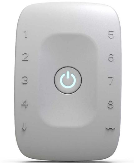
**Figure 3.7:** 8-Channel *biosignalplux* kit
