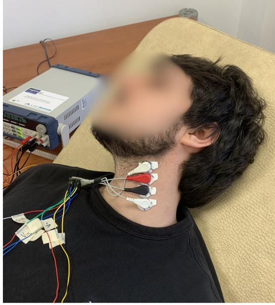
**Figure 6.6:** IPG electrodes placement: the excitation electrodes are the outer coloured of white, while the sensing electrodes are the inner red and black.
