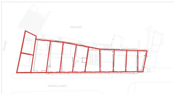
Figure 67: Proposed schematization and simplification of the structural layout for the four levels of the structure.
