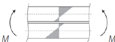
Figure 2-22: Stress profile due to bending stresses in case of partial composite effect 27 .
