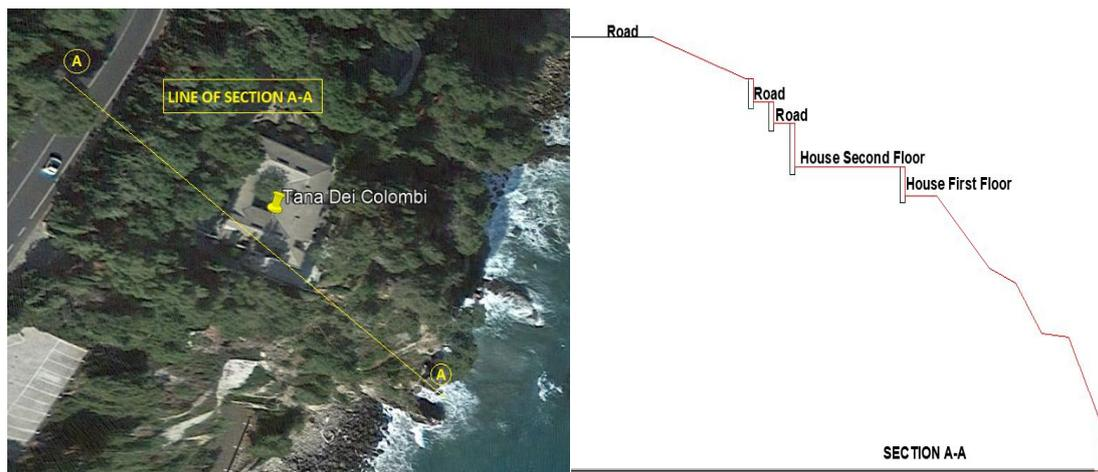
Figure 3.2.2.1 Line of Section & Section A-A considered for analysis
