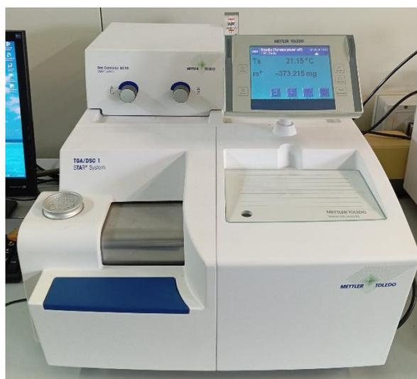
**Figura 4.4** TGA Mettler Toledo
