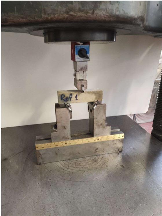
Figure 32 Ref\_1 sample before the test
