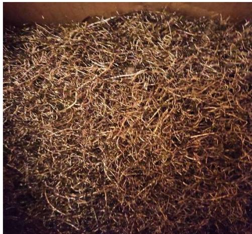
Figure 17 steel fibres from AGR
