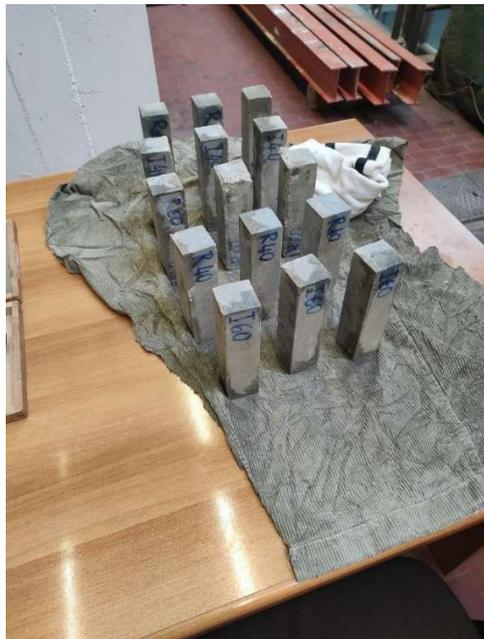
*Figure 30 samples after 28 days of curing*
