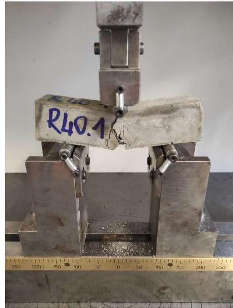
Figure 33 R40\_1 sample after failure
