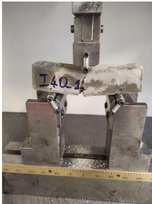
Figure 35 I40\_1 sample at failure
