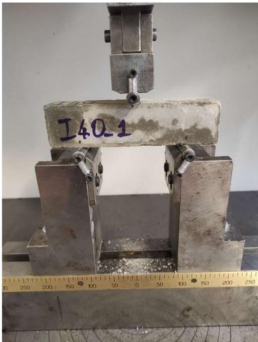
Figure 36 I40\_1 sample before testing
