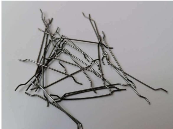
*Figure 13 steel fibers*
