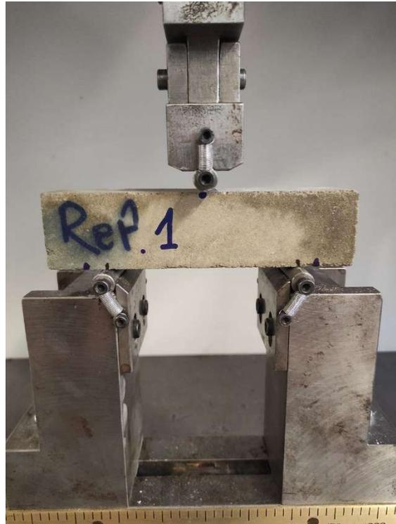
Figure 31 Ref\_1 sample after failure
