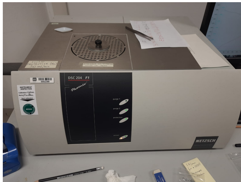
Figure 2.2: DSC instrumentation used.
