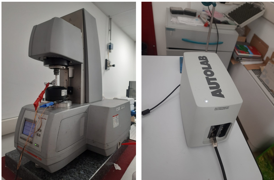
Figure 2.8: Setup for PEIS analyses: on the left, the rheometer attached to the potentiostat to the right.
