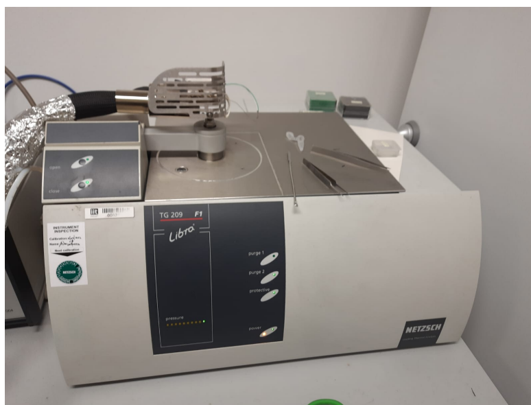
Figure 2.1: TGA instrumentation used.
