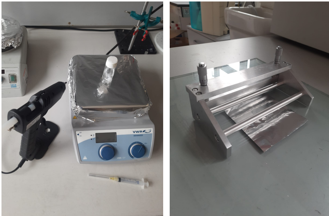
Figure 2.9: On the left, the setup for the production of the ionogel solutions; on the right, the Dr.Blade used for casting.
