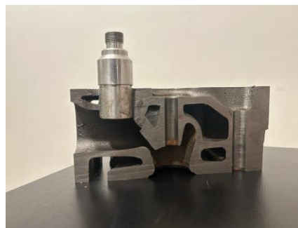
Figure 19 - Section Of The Engine Head with The Installed Spark Plug Seat
