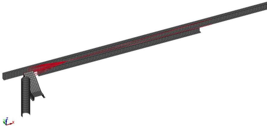
Figure 3: Section on the model in the XZ middle plane. The nodal rigid constraint is displayed in bright red.
