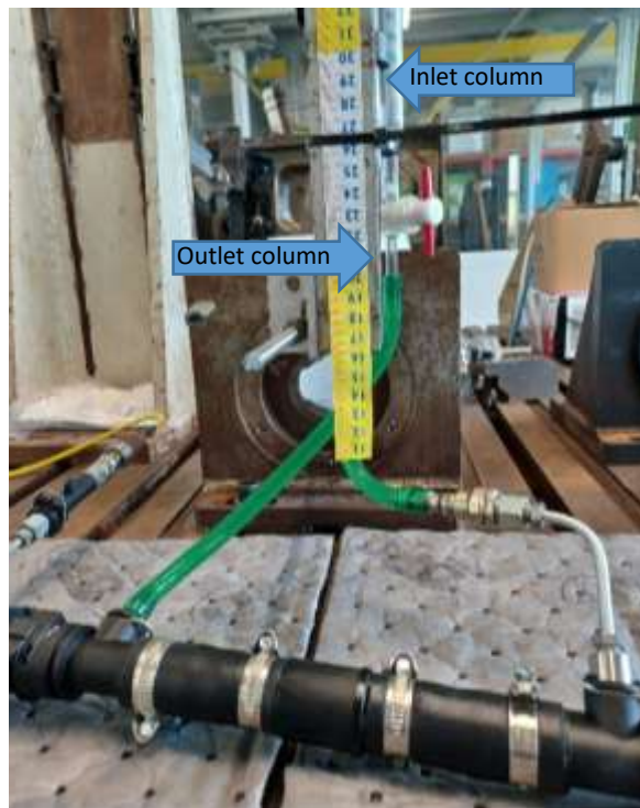
Figure 2-5: Pressure drop test setup
