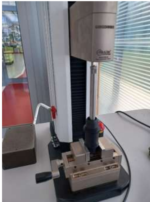
Figure 2-16: Spring testing with loadcell
