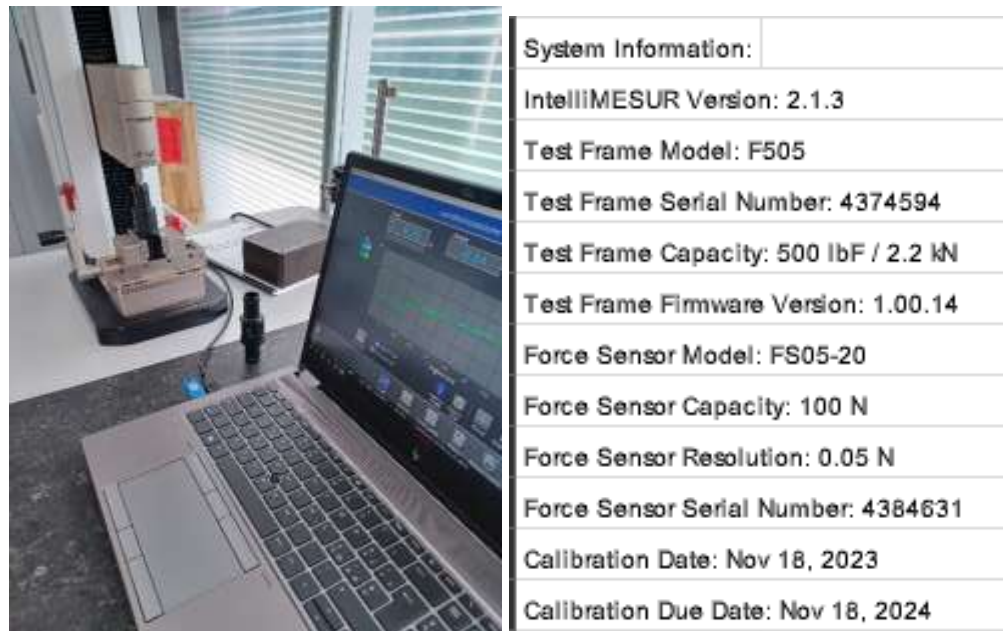
Figure 2-14: (a) Loading cell “ Mark10 ” and (b) system information
