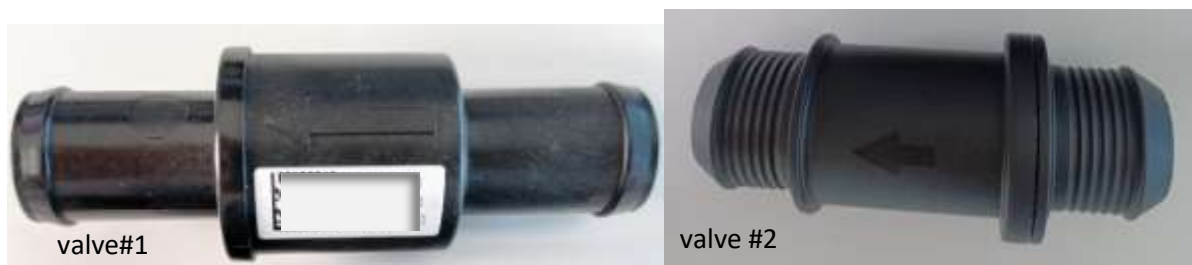
Figure 2-1: Physical check valves under testing
