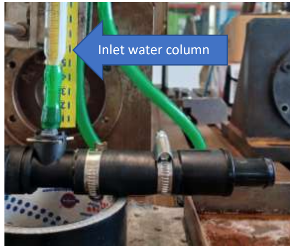
Figure 2-20: Cracking pressure through water column method
