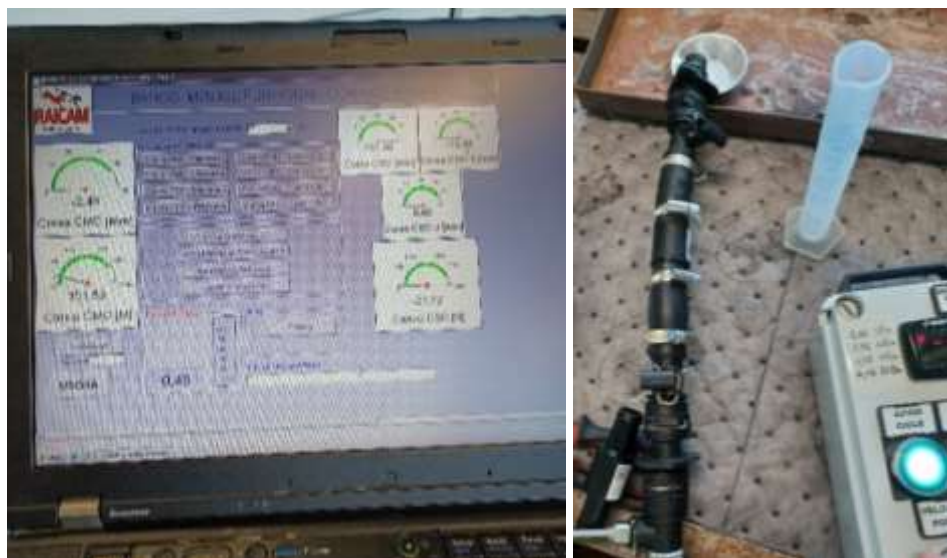
Figure 2-11: Pressure measurement and backflow test
