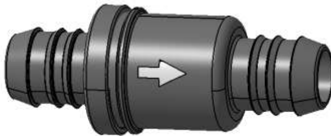
Figure 1-3: Example of unidirectional valve CAD model
