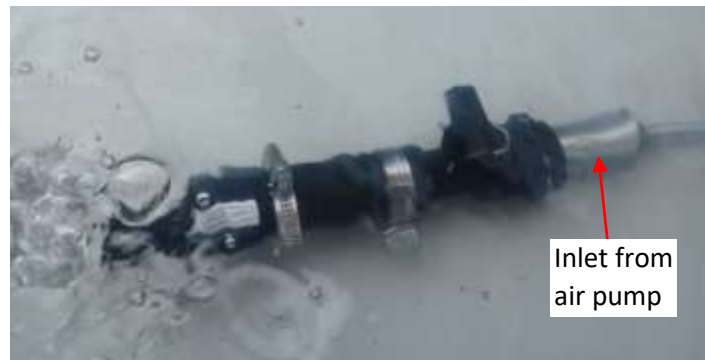
Figure 2-19: Air-water cracking pressure test
