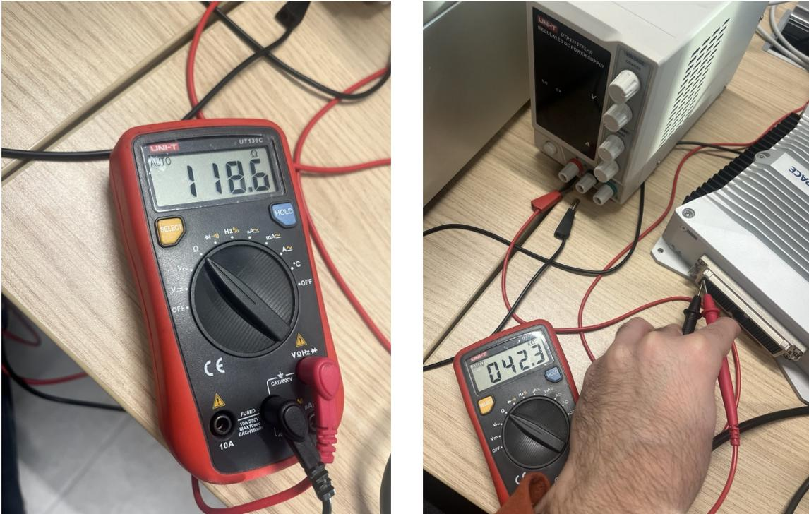
Figure 42: Multimeter: resistance measures
