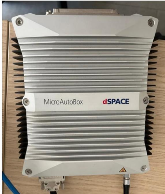
Figure 12: dSPACE MicroAutobox III Hardware
