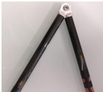
**Figure 2.2:** Strain gauge on a suspension arm
