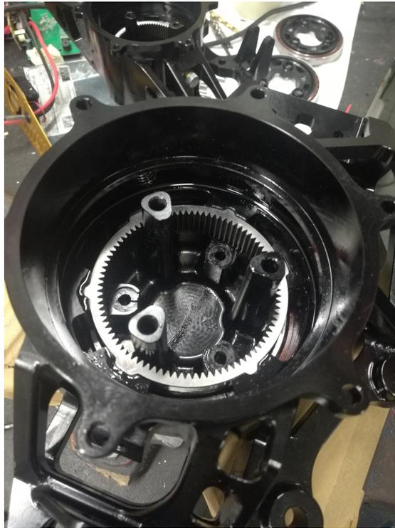
**Figure 2.5:** Upright's inner part with only the ring gear, the hub, and the bearing with its oil seal (cannot be seen from this angle). In the front are the holes and the face that connect the motor plate.
