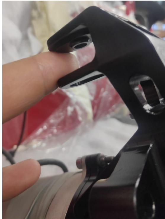
**Figure 2.6:** A flip-chip mounted on the upright, we can see the loop shape of the component.
