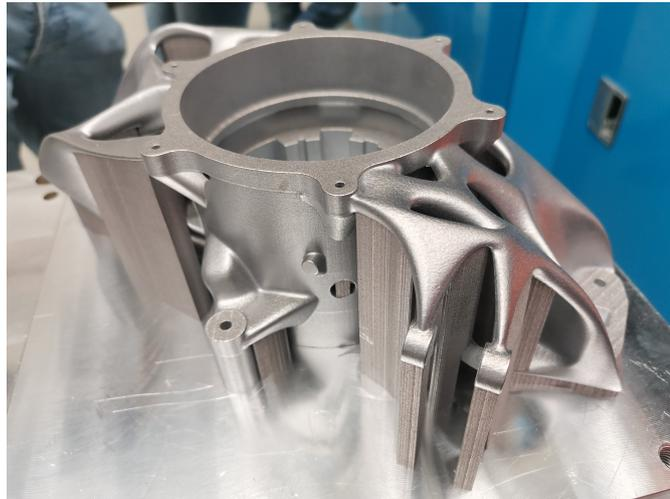
**Figure 2.1:** The SC21 upright after the 3D printing.
