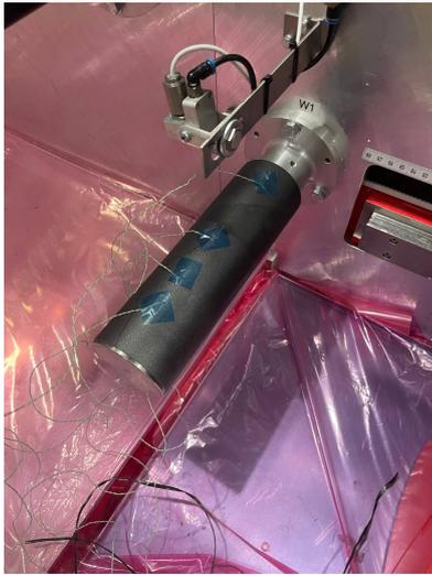
Figure 2.6 : Thermocouples attached to first fulling roller's surface
