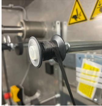
Figure 2.12 : Fiber damage on a cross-winder roller
