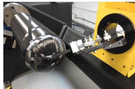
Figure 1.2 : Towpreg winding. Retrieved from TCR Composites
