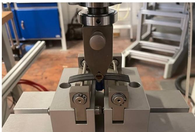
Figure 2.14 : Curved beam bending test setup
