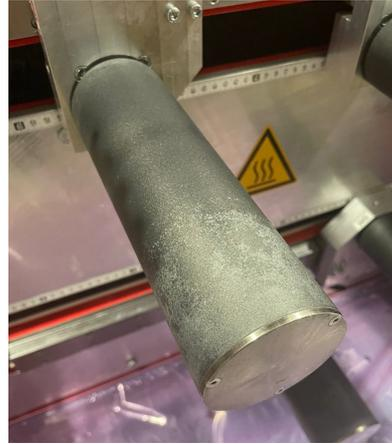
Figure 2.7 : Fulling roller surface abrasion
