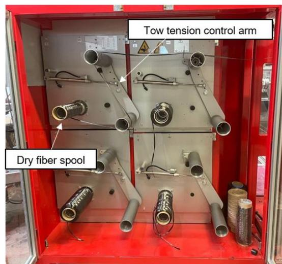
Figure 2.2 : Dry fiber spools unwinding section
