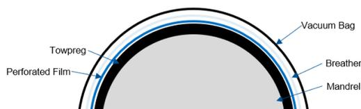
Figure 3.5 : Setup of the vacuum bagging of the cylinders
