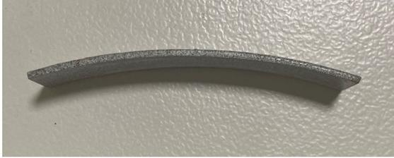
Figure 3.9 : Curved beam bending test sample
