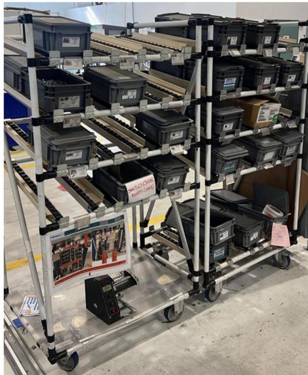
Figure 5.1: New rack configuration for components at Ass.P6
