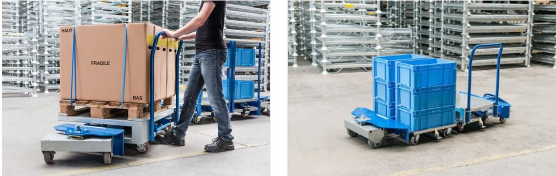
Figure 5.10: Example of Tow Train for Milk-Run
