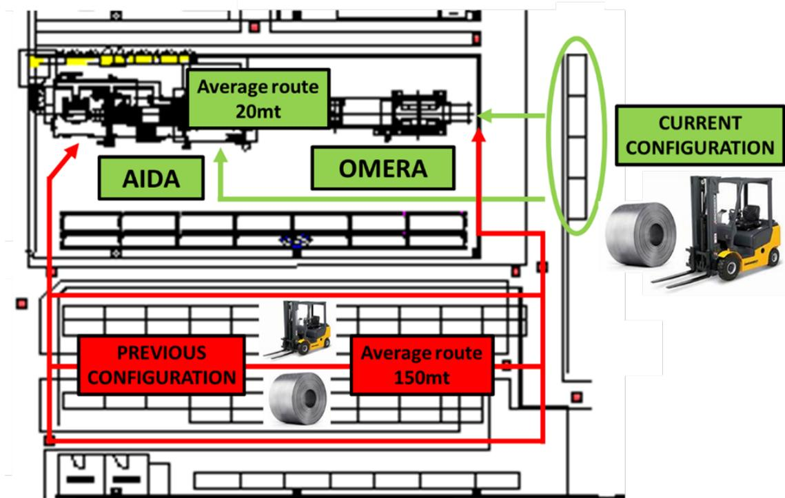
Figure 3.19: Aida and Omera: Re-design of routes and allocation of Coils
