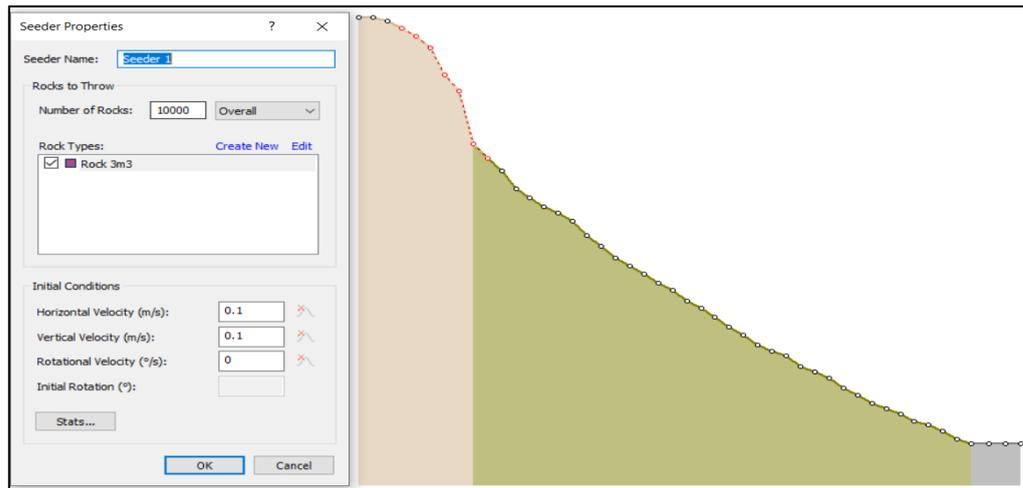
*Figure 5.5.1 Location of Line seeder in the slope profile made in Rockfall 2*
