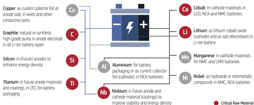
Figure 3. Raw material used in batteries [37]
