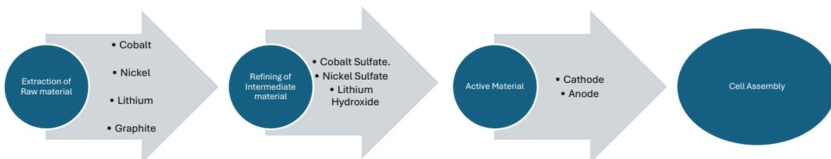
Figure 2. Streamlined representation of the battery cell product system
