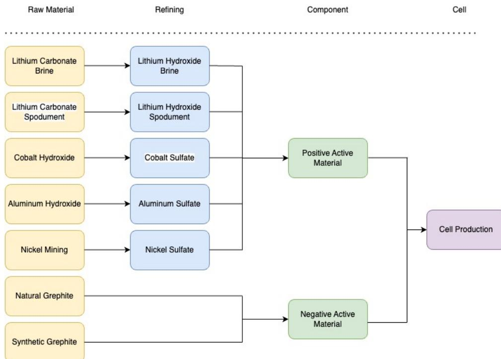
Figure 10. Cradle-to-gate product system for NCA lithium-ion batteries [32]
