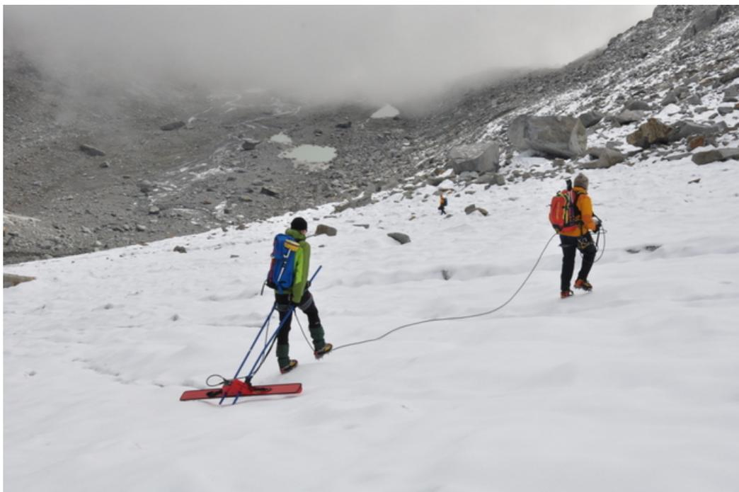
*Fig. 15 - Ground Penetrating Radar (GPR) prospecting for the determination of the thickness of the Ciardoney glacier, by Imageo Srl (f. SMI)*
