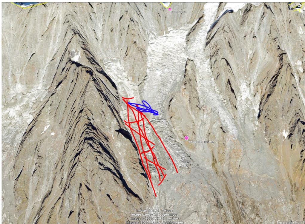
Fig. 32 - Original GPR lines available; data of Planpincieux 2019 are red, while data of Planpincieux 2021 are blue.
