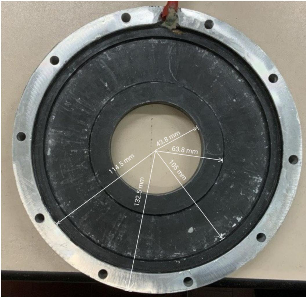
Figure 2.3: Geometric dimension of the stator
