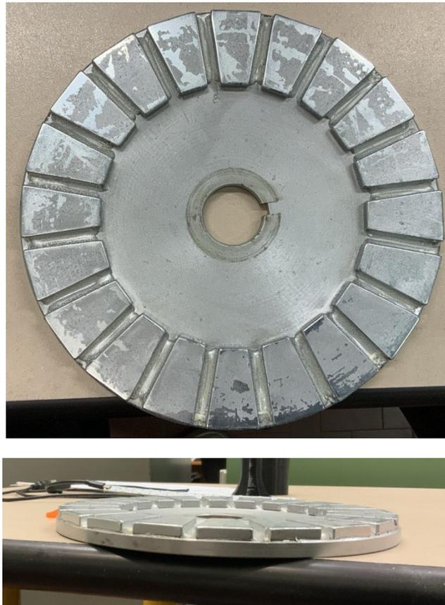
Figure 1.5: The rotor of AFPMS actual generator under study
