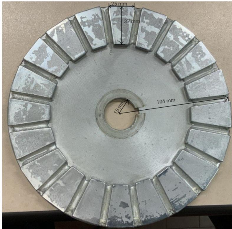
Figure 2.5: Geometric dimension of the rotor
