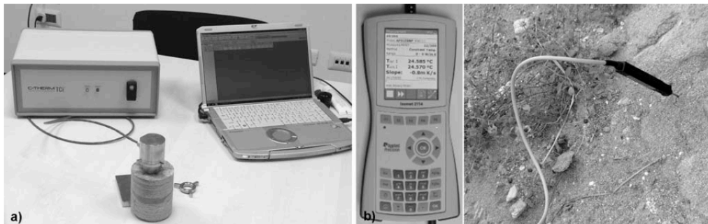
Figure 19: Thermal conductivity analyzers composed of interfacial sensor and central unit operating following the modified transient plane source method (a) and the transient line source method (b) (19).
