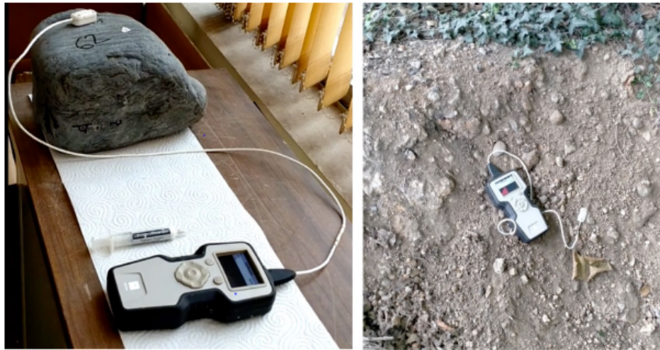
Figure 26: Measurement of thermal conductivity by means of a Tempos thermal needle probe device on a boulder sample using a rock sensor (RK-3) and thermal grease (left) and on clayey alluvial sediments using a soil sensor (TR-3) in situ (right) (27).
