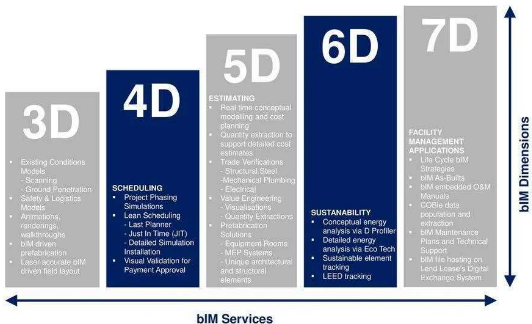
Figure 4.16: BIM Dimensions, Eleftheriadis, 2014
