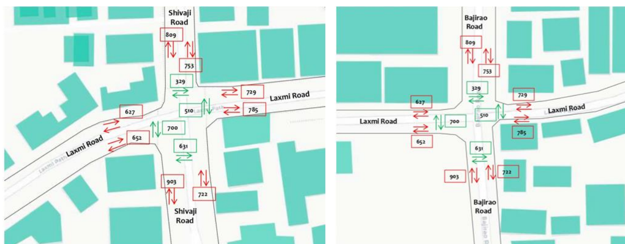
Figure 57 - Schematic pedestrian count in Belbaug Chowk and Nagarkar Talim Chowk (Source - CMP, 2018 modified by author)
