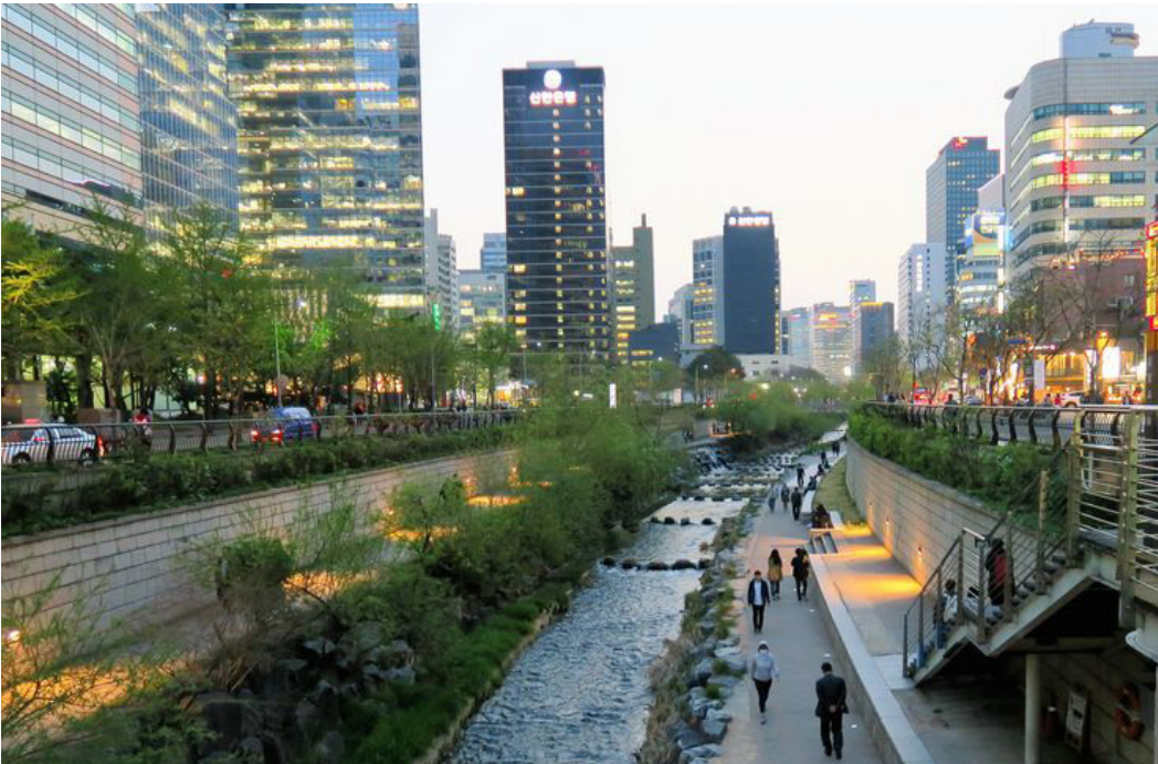
Fig.24: Natural stones are used to both create walkways for pedestrians and to help regulate water speeds and levels and various points along the stream. © Alamy Stock Photo
