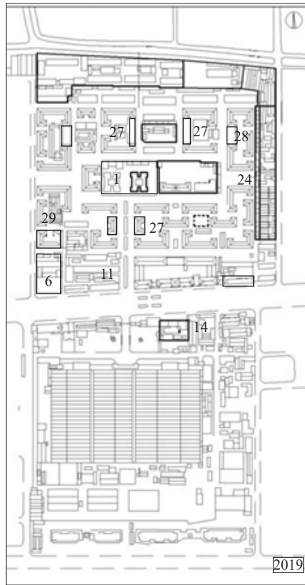
Figure 3.3-2. Using Beijing 2nd Cotton Textile Factory as an Example. This illustrates the spatial changes of Chinese danwei. It is evident that building density has increased, and large-scale buildings and plazas have been demolished.
