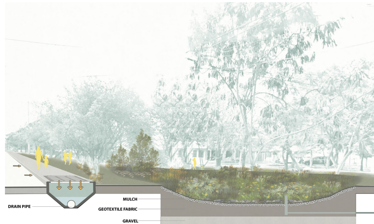
Figure 162 Roadside planting detail section (Source: Illustration by Authors)
