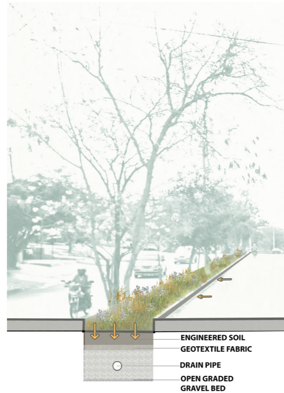
Figure 162 Roadside planting detail section (Source: Illustration by Authors)
