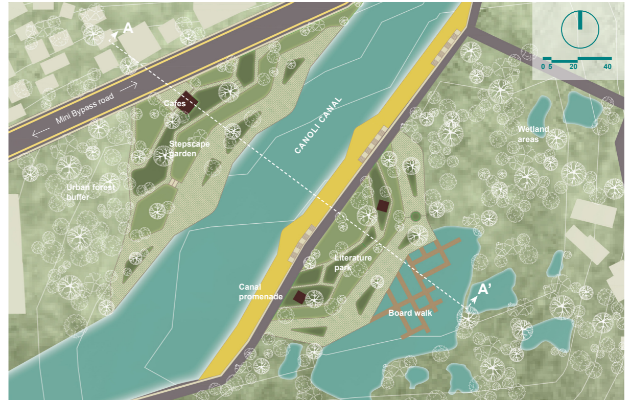
Figure 139 Schematic plan showing activity layouts of the recreation zone (Source: Illustration by Authors)
