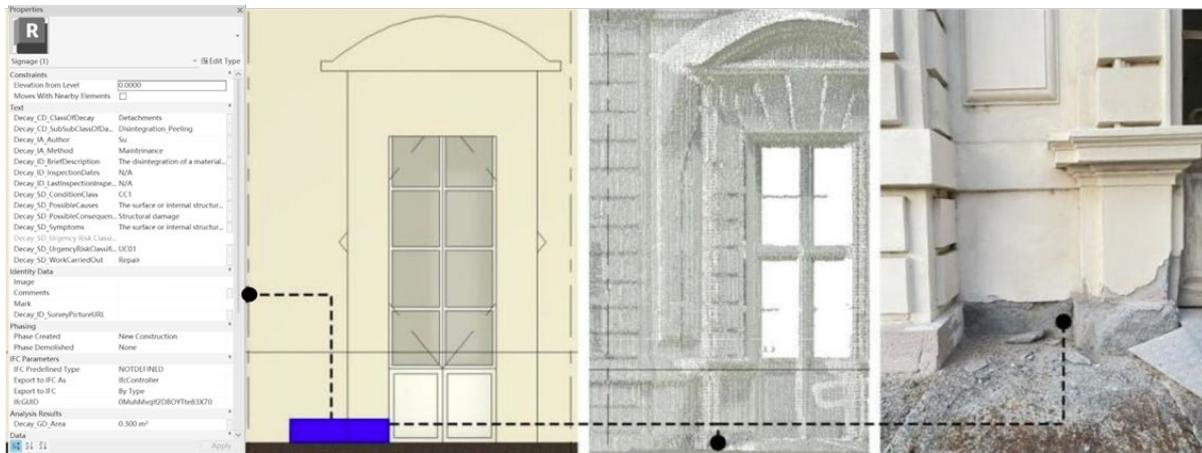
Figure 37 Spalling represented using patch-type objects (in-situ components/identifications) in blue.
