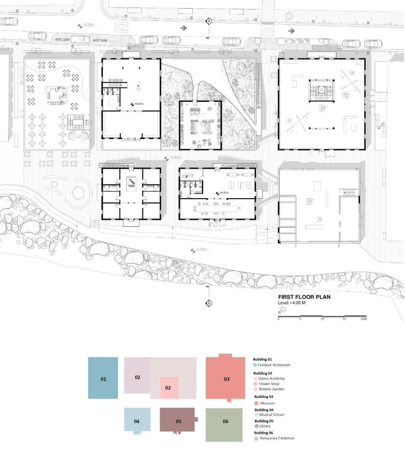
Figure 214. First Floor Plan of The Selected Historical Buildings, Illustrating Adaptive Reuse Strategy , and Highlighting Their New Functions (N.Maawad, A.Khoury)
