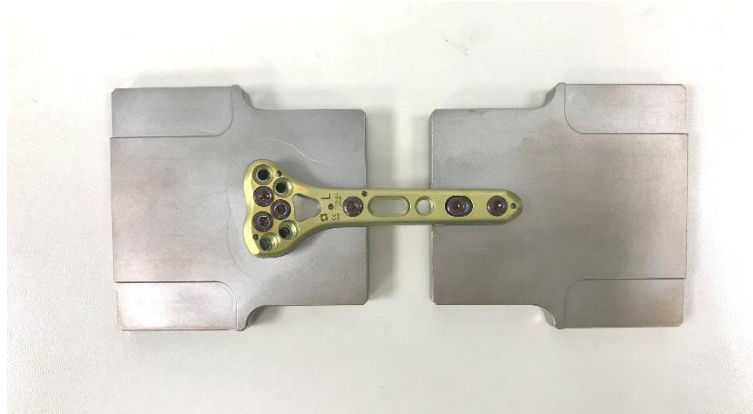
Figure 1: Pre-Test Specimen for Static 4-Point Bending
