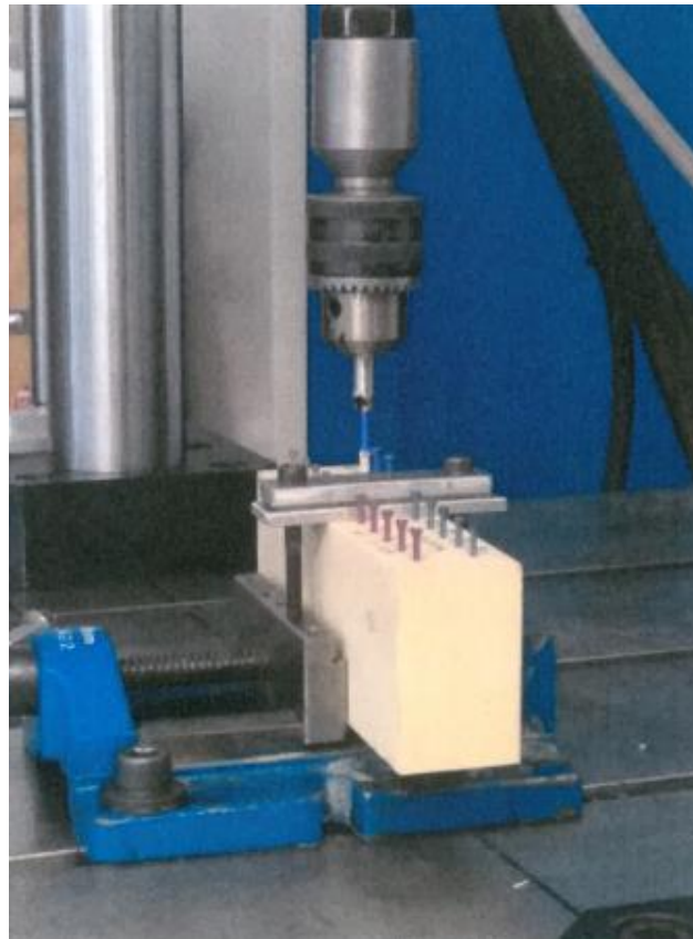
Figure 5: Pull-Out Test Set-Up
