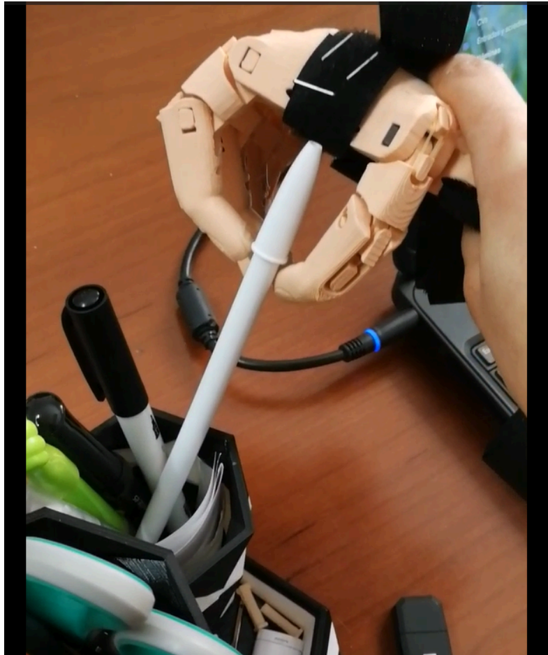
Figure 2.1. Example of precise three-digital grasp performed with a Nelly, form Ayúdame 3D
