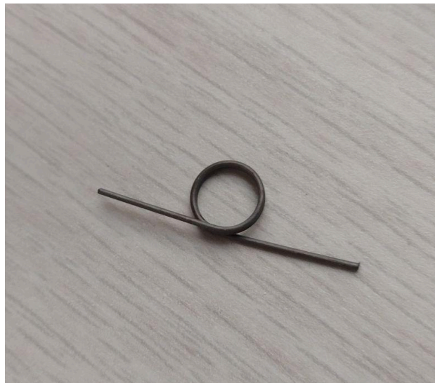
Figure 4.3, Photo of the torsion spring to be inserted between the phalanxes
