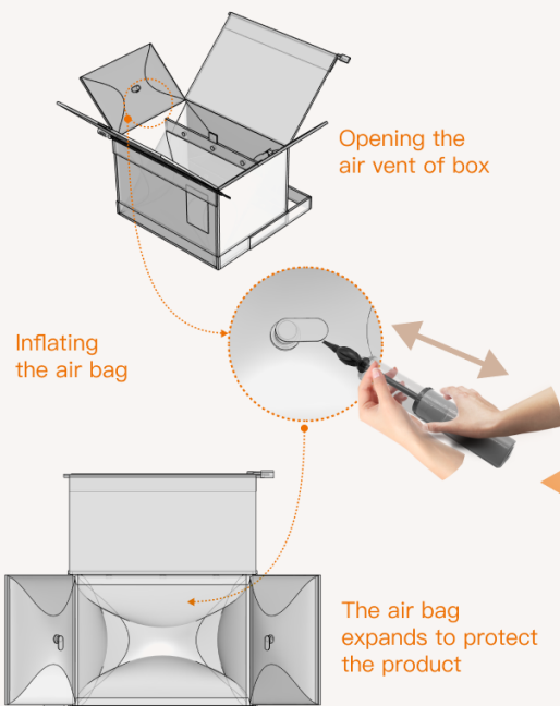
Figure 6-4. Reusable express packaging box structure drawing Drawn by the author
