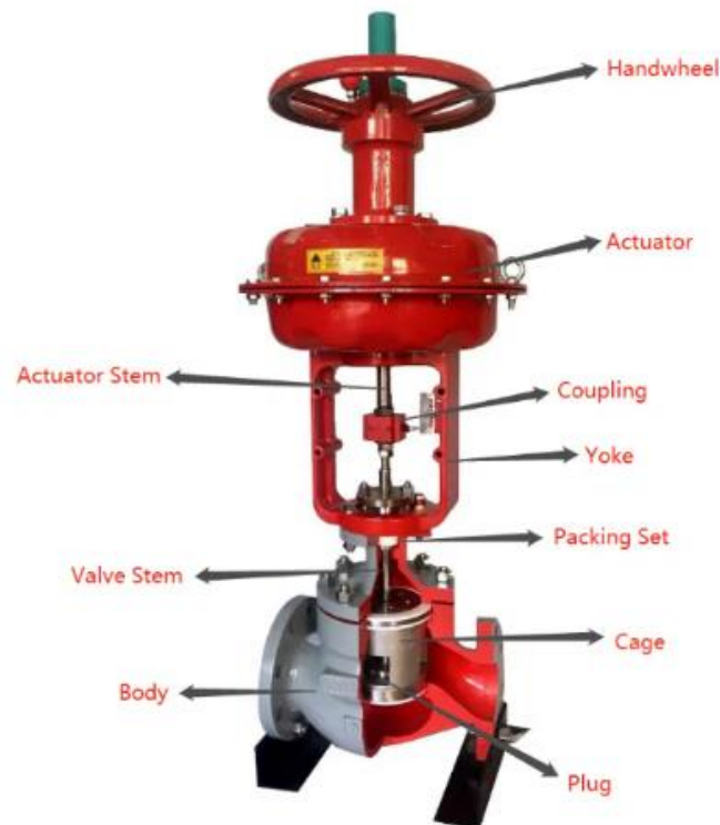
Figure 1.7 Control valve components (Don, 2022)
