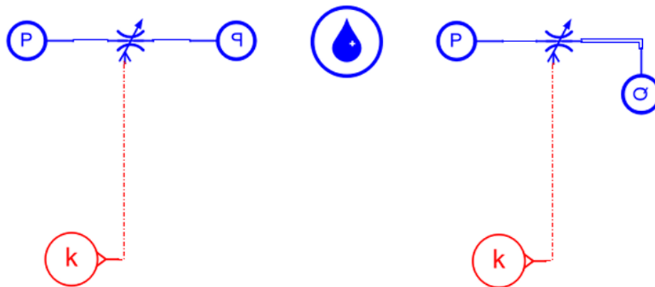
Figure 2.3 Case P-P: Pressure Inlet-Pressure Outlet (left) and Case VFR-P: Volume Flow Inlet-Pressure Outlet (right)
