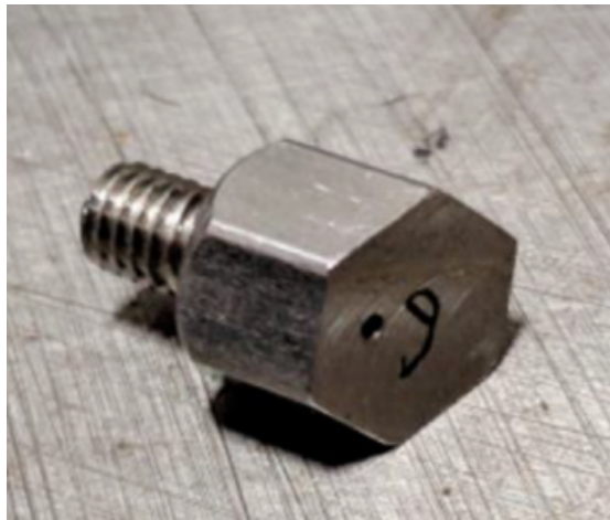
Figure 5.12: One of the swirl injectors manufactured by previous students at Cal Poly
