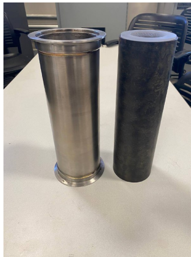
Figure 5.16: Grain inserted in a liner next to the combustion chamber
