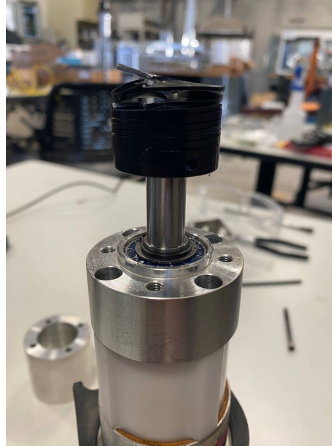
Figure 4.18: Image of the coupling fracture after the DC motor was removed from the system
