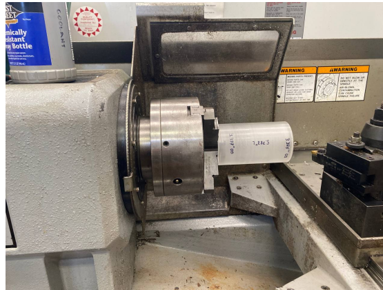
Figure 5.15: Half grain on a CNC Lathe before its OD is turned
