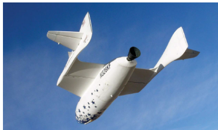
Figure 1.3: StarShipOne during glide down. The propellant for this configuration is HTPB-N 2 O
