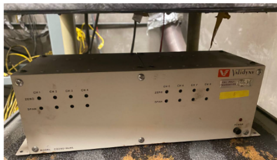
Figure 4.12: Demodulator that connects PTs to DAQ. The two holes for each channel hide the screws that are used to adjust gain and zero for each sensor
