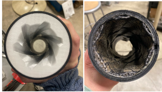
Figure 6.10: Visual comparison of the helical grain geometry before and after the hot test
