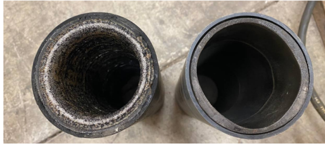
Figure 6.13: Visual comparison of the two baseline grains. On the left the 3D printed grain, on the right the traditionally machined
