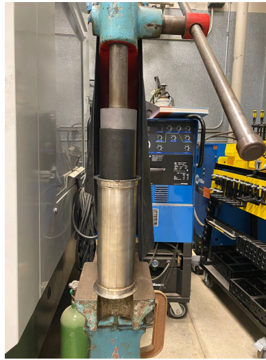
Figure 5.17: Grain-Liner assembly being press fit into the combustion chamber
