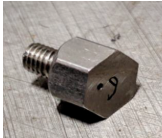
Figure 6.7: Swirl injector before being mounted into the pre chamber
