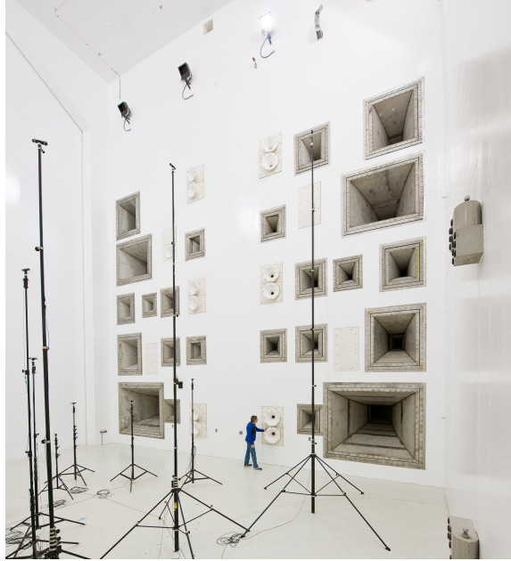
Figure 3.7: Reverberant Acoustic Chamber [15].
