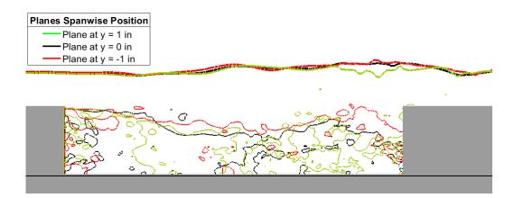
Figure 3.14: Boundary layer and reverse flow region comparison.
