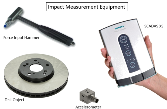
Figure 3.1: Hammer testing set-up[17]
