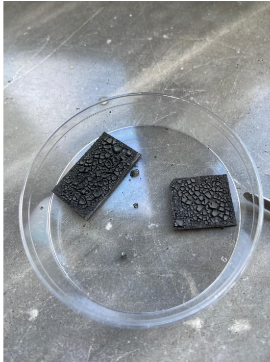
Figure 4.2: Coated SiC/SiC with pure Tethon 3D slurry (TT1 and TT2)
