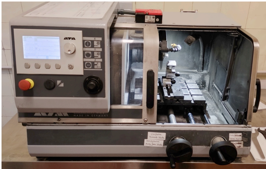
Figure 5-1 Brilliant 220 cutting machine
