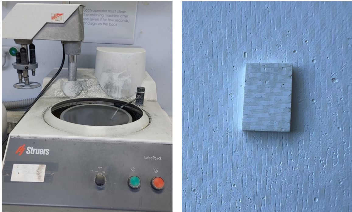
Figure 5-2 a) Labo-pol 2 b) polished substrate in front, unpolished in the back
