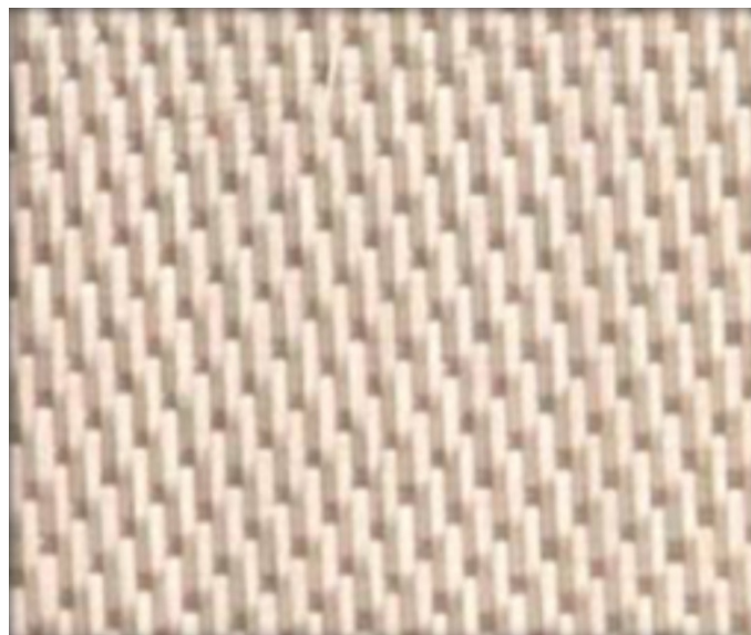
Figure 4-9 Visual appearance of the Nextel 610 fiber fabric [66]
