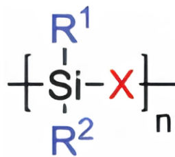
Figure 3-4 Simplified molecular structure of organosilicon compounds [31]
