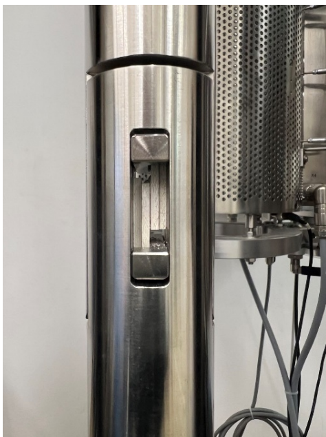
Figure 5-7 On left the specimen grip with sample pre-test, on right the design dimension for the specimen [67]
