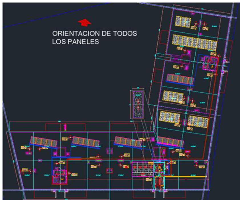
Figure 30: Optimal orientation of the panels, on AutoCAD.
