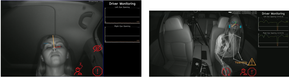
Figures 11 & 12: Examples of sleepiness (image 11) and yawning (image 12) detected by DMS
