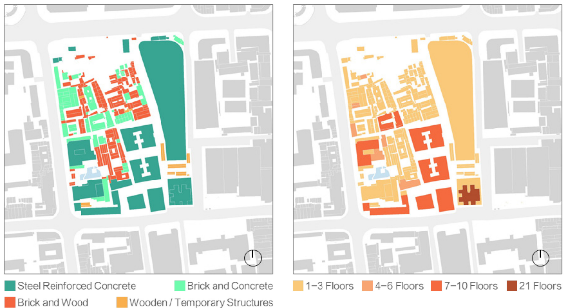
Figure 5-15 Current Condition of Building Structure
