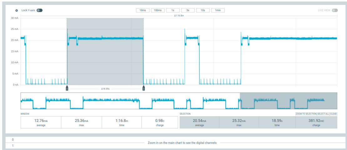
Figure 5.17: Power consumption graph for STM32U575 obtained using PPKII
