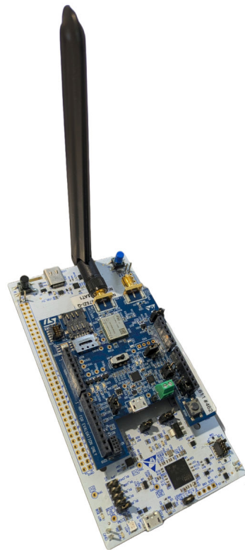
Figure 4.17: EVLST87M01 placed on top of the NUCLEO-U575ZI-Q Nucleo development board
