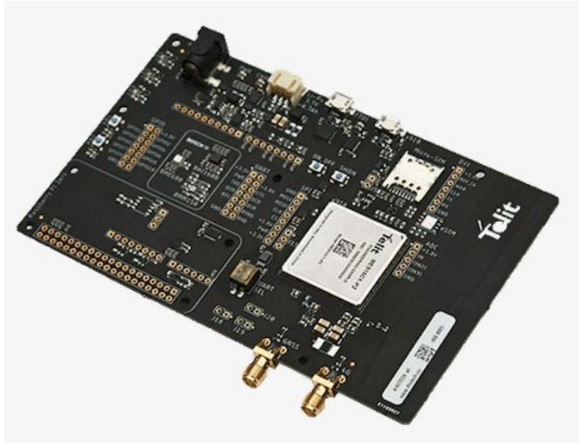
Figure 3.3: Telit Bravo development board [17]
