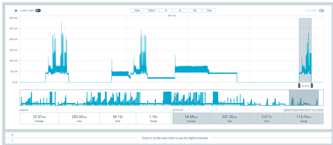
Figure 5.18: Power consumption graph for the STEVAL-NBIOT obtained using PPKII
