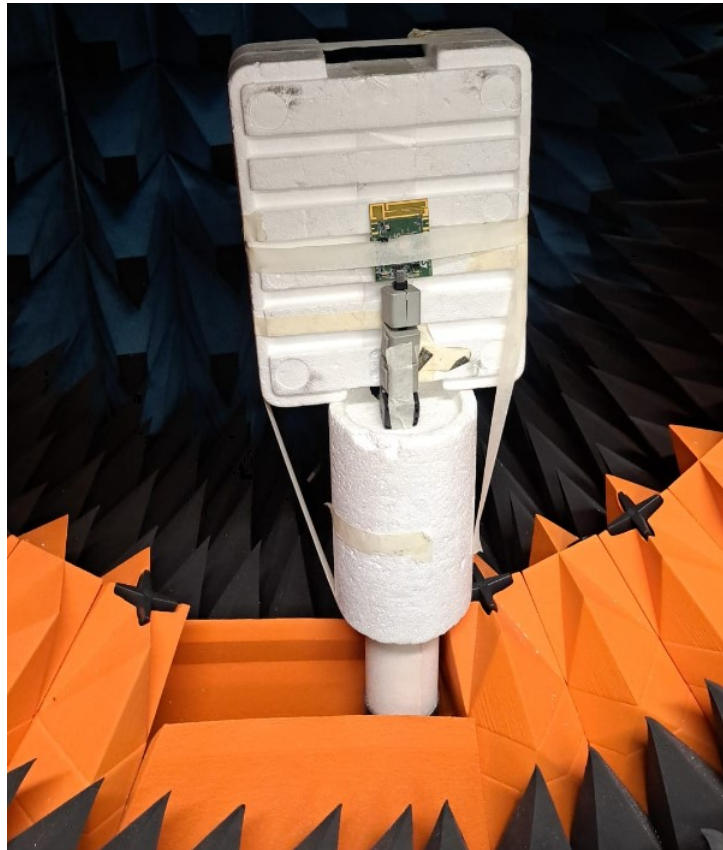
Figure 5.1: Test environment for evaluating the NB-IoT antenna performance of the STEVAL-NBIOT
