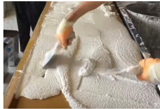
Spreading the mixture into the mold with the help of spatula
