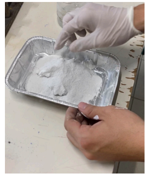
Third step, preparation of the materials for the second mixture (outer layer); plaster, marble dust, water (Kamis 2024)
