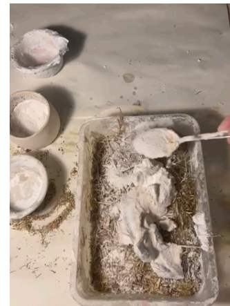
Adding marble dust to the mixture (Kamis 2024)
