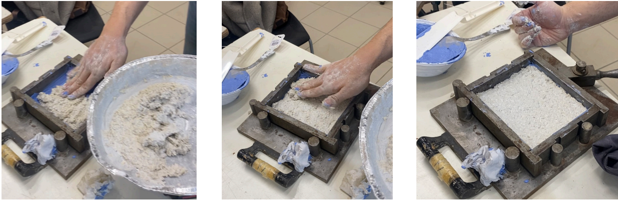
Seventh step, pouring the first mixture as the main layer and leaving to dry at room temperature (Kamis 2024)
