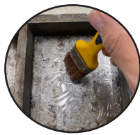
Preparing the mold; applying the oil
