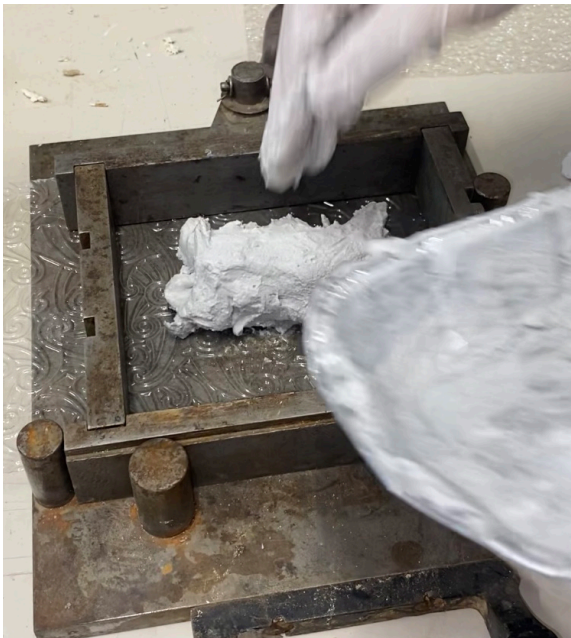
Sixth step, pouring the second mixture as the outer layer (Kamis 2024)
