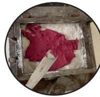
Pouring the mixture of aesthetic outer layer, Tadelakt
