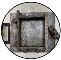
Preparing the mold; placing a pattern
