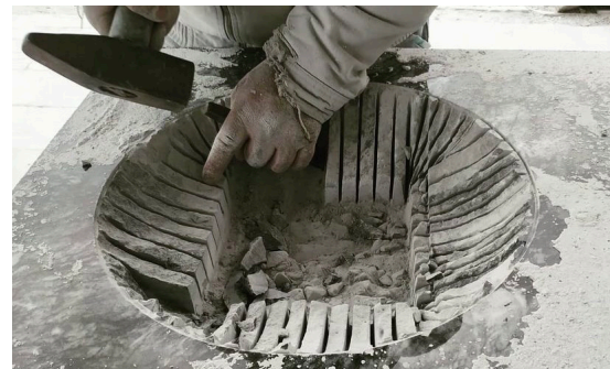
Second step, breaking the striped part (Bağcı 2019)
