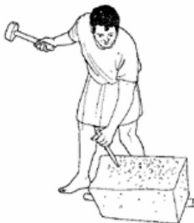
Image of a stonemason processing a stone block with the help of a hammer and chisel (Adam 1994)
