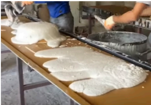
Seventh step, pouring the mixture into the mold and spreading
