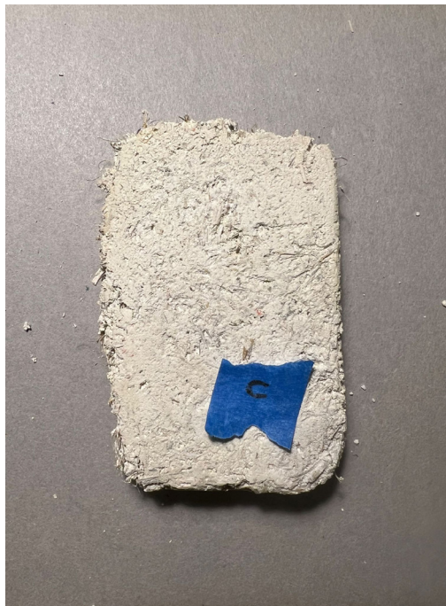
The back surface of sample 1C which was polished with soapy water after drying (Kamis 2024)
