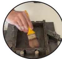
Preparing the mold; applying oil
