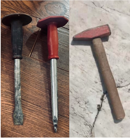
Mason chisel and hammer used to take samples from rocks (Kamis 2024)
