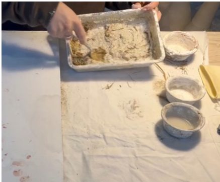
Second step, mixing the mixture, pouring into mold and leaving to dry at room temperature (Kamis 2024)
