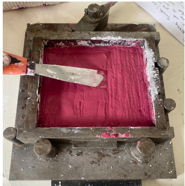
Seventh step, pouring the second mixture as Tadelakt, creating the pattern on it and leaving to firm up at room temperature (Kamis 2024)
