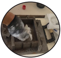
Preparing the mold; applying oil
