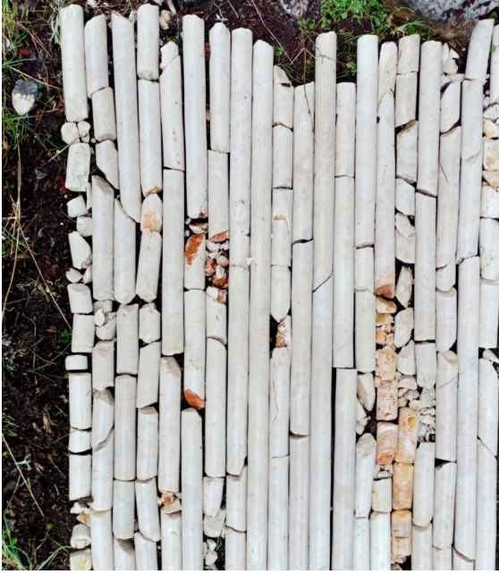
From the research carried out in Kumluca, marble samples taken by using the core drilling machine, Antalya, Turkey (Çal 2023)
