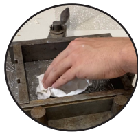
Preparing the mold; applying oil
