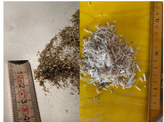
Hemp particles obtained by sieving the hemp hurd (Kamis 2024)
