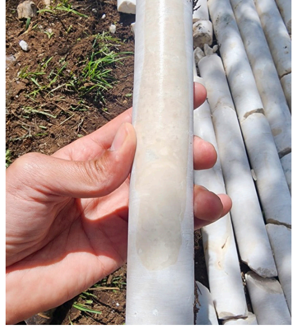
From the research carried out in Kumluca, marble samples taken by using the core drilling machine, Antalya, Turkey (Çal 2023)
