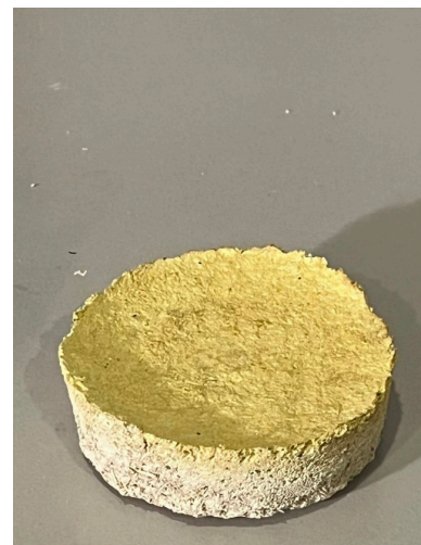
Second step, mixing the mixture, pouring into mold and leaving to dry on the heater (Kamis 2024)
