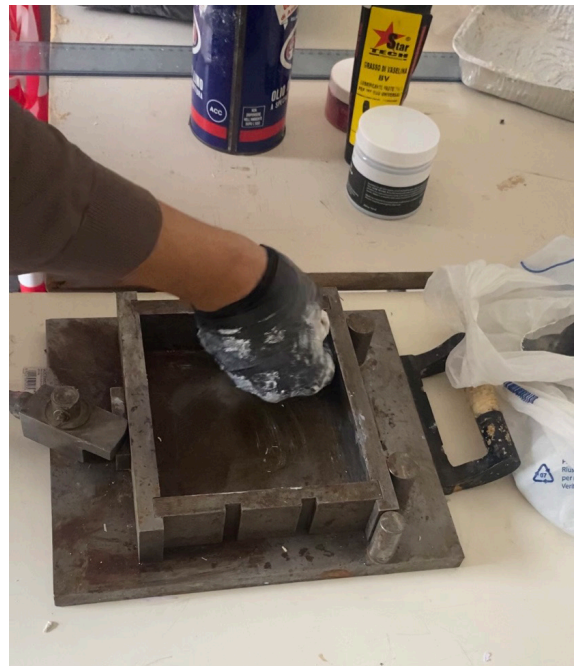
Fourth step, mixing the mixture to obtain Tadelakt as outer layer (Kamis 2024)
