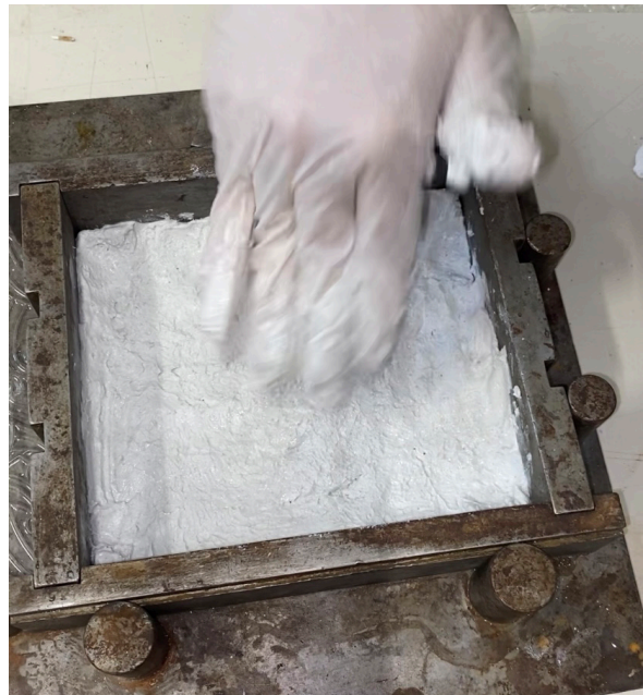
Sixth step, pouring the second mixture as the outer layer (Kamis 2024)
