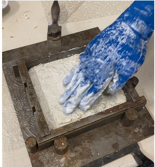
Seventh step, pouring the first mixture as the main layer and leaving to dry at room temperature (Kamis 2024)
