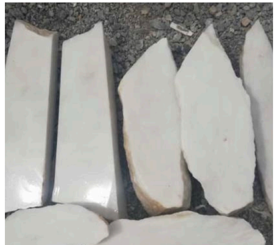
Samples obtained from massive rocks with the help of hammer and chisel for examination (Çal 2024)
