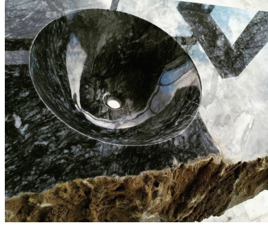
Final step, correcting the form and polishing (Bağcı 2019)
