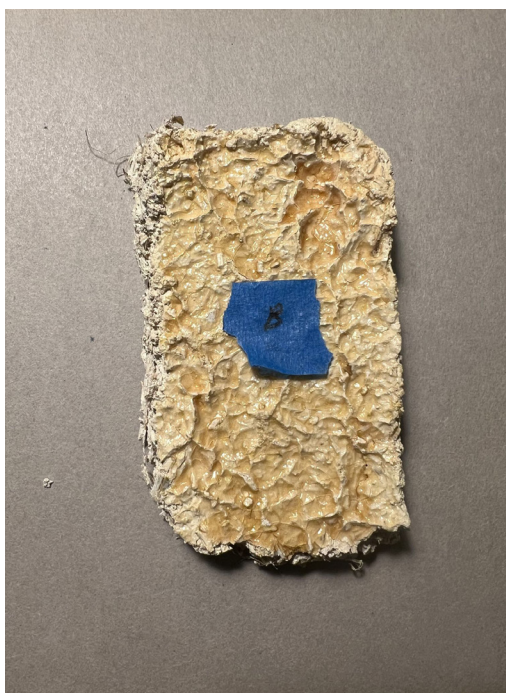
The front surface of sample 1B which was polished with acacia tree resin after drying, the results are the same as in sample 1A (Kamis 2024)
