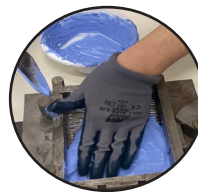
Pouring the mixture of aesthetic outer layer
