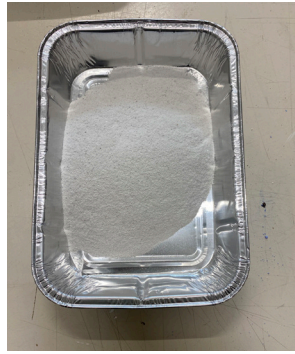
Third step, preparation of the materials for the second mixture (outer layer); plaster, marble dust, water (Kamis 2024)
