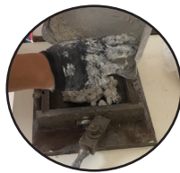
Pouring the mixture of main layer
