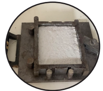
Pouring into mold and leaving to firm up
