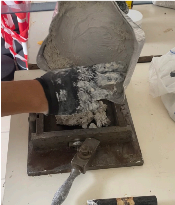
Sixth step, pouring the first mixture as the main layer (Kamis 2024)
