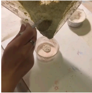
Second step, mixing the mixture, pouring into mold and leaving to dry on the heater (Kamis 2024)
