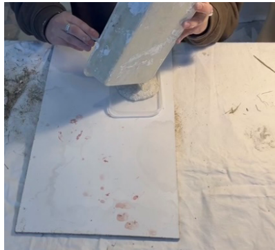
Second step, mixing the mixture, pouring into mold and leaving to dry at room temperature (Kamis 2024)
