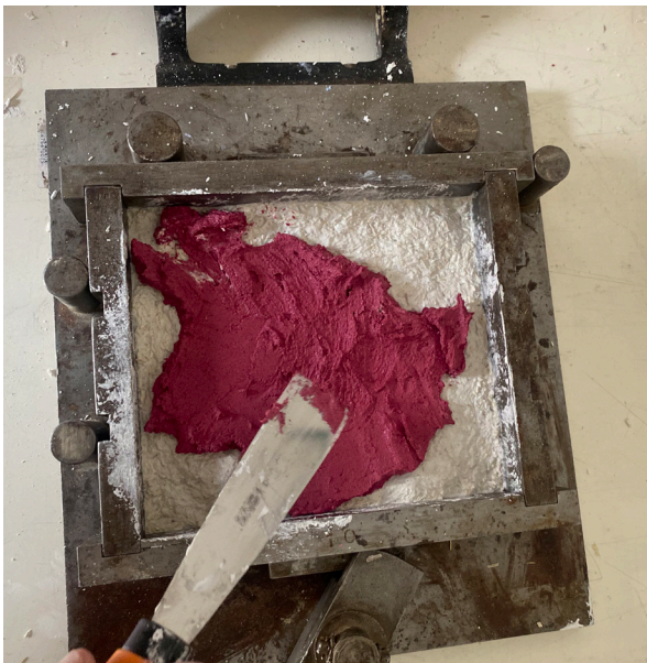
Seventh step, pouring the second mixture as Tadelakt, creating the pattern on it and leaving to firm up at room temperature (Kamis 2024)
