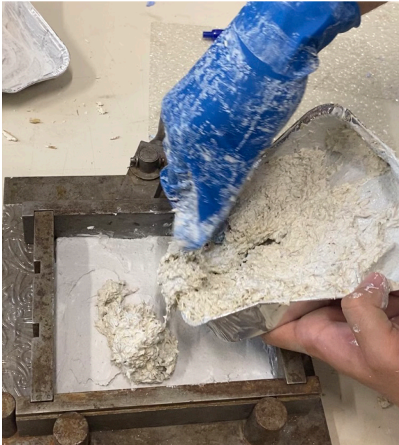
Seventh step, pouring the first mixture as the main layer and leaving to dry at room temperature (Kamis 2024)
