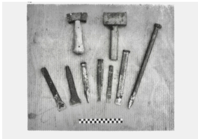
Hammers and chisels used in stone extraction both in the past and today (Adam 1994)
