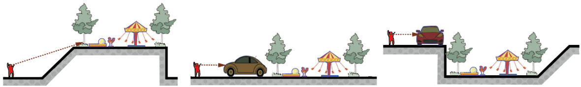
Figure 3-20 The relationship between activity spaces and children's sightlines (Source: Drawn by Author)
